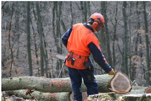
Fig. 18: Fixing the loggers tape at the butt end of the stem (picture: Suchomel, 2010)
